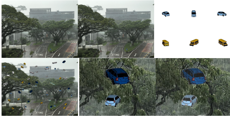
Fig. 2: Examples of vehicle models used in FVR-660 dataset. Top: From left to right are example of an image pair, and the vehicle models used to render on background image. Bottom: From left to right are the rain background rendered with vehicles, and the vehicles without/with applying rain streaks and rain accumulation.
