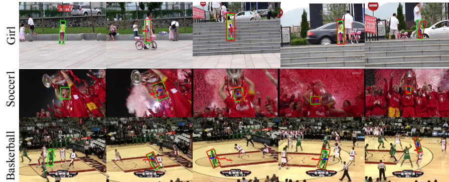
Fig. 5. Qualitative results of Ours-SiamMask for sequences from VOT2018. The red dots denote the target’s past locations and the blue ones are our prediction. In comparison with the groundtruth (green bounding box), our method (red one) performs well under full occlusion in Girl and Soccer1 sequences.
