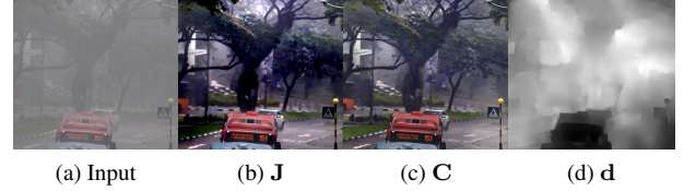
Figure 6: The reconstructed image \mathbf{J} produces darkened result on distant objects. The refinement network restores the details according to normalized depth map \mathbf{d} .
